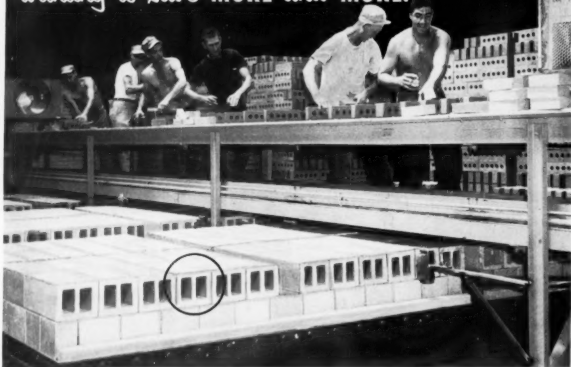
PHOTO—Cloud Ceramics No. 2 Plant, Concordia, Kansas. This modern plant uses 7" x 8 1/2" x 19 1/2" PACO car tops on top deck; 4 1/2" x 8 1/2" x 8 1/4" PACO car tops, with light weight insulation, for perimeter.
